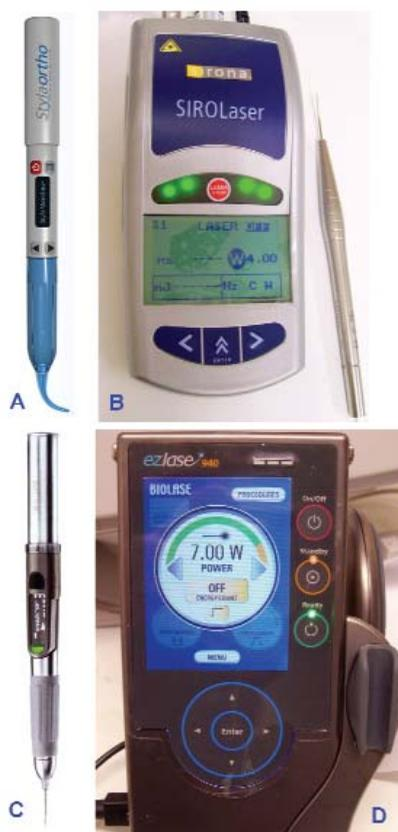
Figure 2. Examples of current diode lasers. A: First generation 810 nm laser (Styla from Zap Lasers) with single patient use rigid fiber. The wireless foot control for this cordless unit is not shown. B: Second generation 980 nm (SIROLaser from Sirona). C: Third generation 940 nm cordless laser with in-built thumb activated switch for laser activation (iLase from Biolase). D: Third generation 940 nm unit (ezlase from Biolase).
