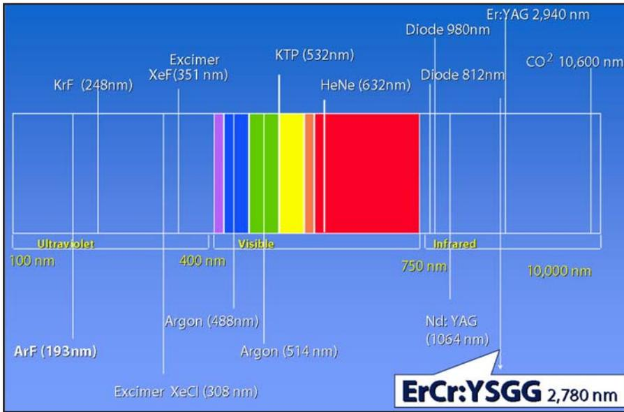
**Fig. 2. Electromagnetic Spectrum.** Lasers have certain properties based on their position in the electromagnetic wave spectrum. The YSGG laser emits a wavelength of 2,780 nanometers, in the mid-infrared spectrum.
