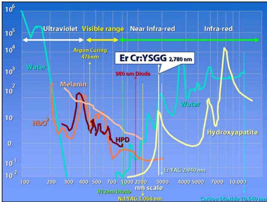
**Fig. 3. Absorption Coefficient Table.** The YSGG laser is near the peak absorption in water, which allows it to effectively cut enamel, dentin, hydroxyapatite and bone. Despite their proximity on the scale, the Er,Cr:YSGG and Er:YAG are separated by more than 300% on the scale.
