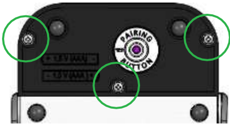
Figure 9.7 Battery cover screws.
