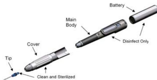
Figure 6–1: Disassembly for Disinfection, Cleaning, and Sterilization
