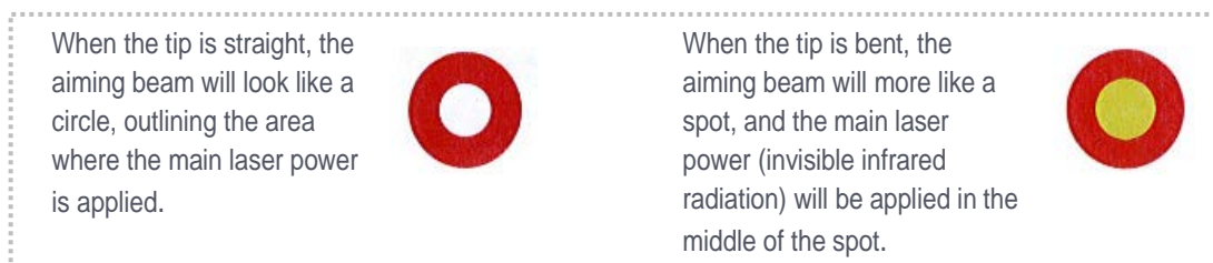
Figure 4-3: Aiming beam pattern.
