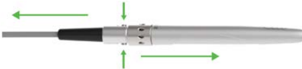
Figure 7.3: Disconnecting the Handpiece from the Fiber Optic Cable
