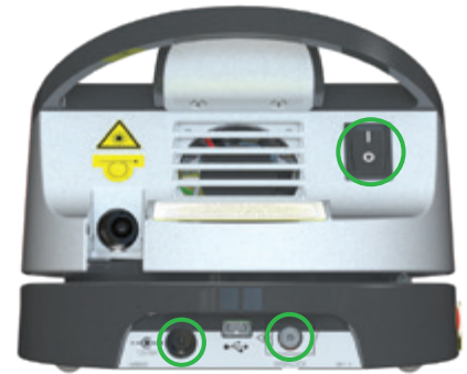
Figure 6.1: Power Switch, DC Power Input, Remote Interlock
