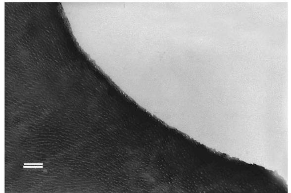
**FIG. 2.** Representative light microscopic photograph from group 1-a. Linear edge without undulation was observed. No caries affected substance or thermal effects were observed (original magnification,  $\times 200$ ; bar represents 30  $\mu\text{m}$ ). D-score was 9.
