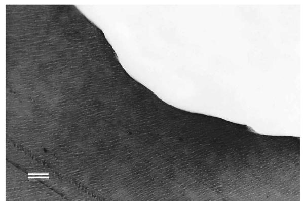
**FIG. 3.** Representative light microscopic photograph from group 2-a. Edge was shaped in mild undulation with a step. Very smooth cutting margin was observed (original magnification  $\times 200$ ; bar represents 30  $\mu\text{m}$ ). D-score was 26.
