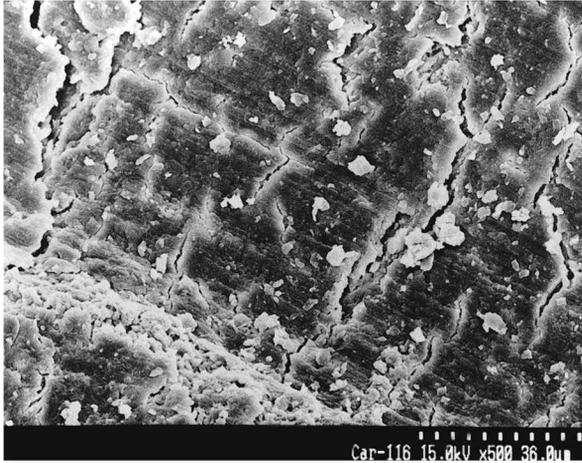
**FIG. 8.** Representative SEM photograph from group 1-b. Finishing treatment removed much debris, but smear layer and some debris were still observed (original magnification,  $\times 500$ ; bar represents 36  $\mu\text{m}$ ). D-score was 8.
