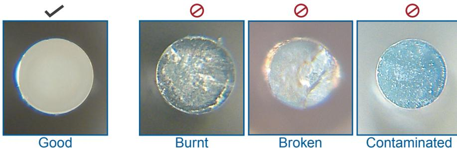
6. Remove the Tip from the test holder using the Tip Remover. If the Tip is contaminated at either end, try cleaning it as shown below. If the Tip is damaged, replace it from the Handpiece using the Tip Remover and dispose of it.
